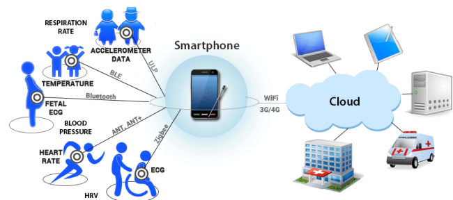
Fig. 2 Framework for remote patient monitoring system, with smartphone as a processing tool
