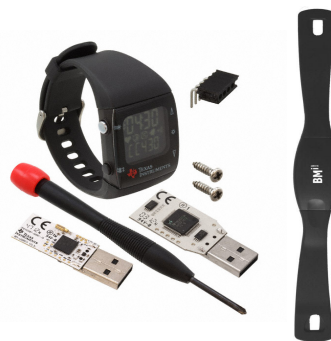
Fig. 2 Texas Instruments EZ430 Chronos watch and BlueRobin Heart rate monitor
